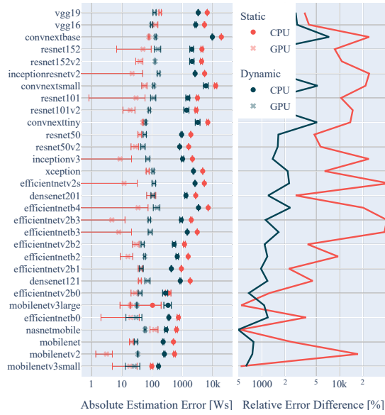
Figure 6: Absolute energy estimation errors of vision models when deployed on the CPU or GPU (left). Both the static and dynamic approaches make higher errors for CPU inference, and the differences between the CPU and GPU errors (right) grow with model complexity.
